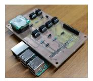
The PUF itself is ad-hoc hardware, fabricated through the EUROPRACTICE Consortium, connected to a Raspberry Pi board by means of a signal-levelling custom interfacing printed circuit, connected to the expansion pins. We leverage the board's already available software substrate for the other components.
